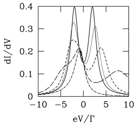
FIG. 3. Differential conductance  $\partial I/\partial V$  in units of  $(1 - \Gamma^A/\Gamma)e^2/h$  for a quantum dot with  $\eta = 0$ ,  $\Gamma^L/\Gamma^R = 3$ , and  $\Delta\epsilon/\Gamma = 1$  ( $Q_G = 0$ ) for  $C_A/C_\Sigma = 0$  (solid curve);  $1/4$  (dotted curve);  $1/2$  (short dashed curve);  $3/4$  (long dashed curve);  $1$  (dash-dotted curve). Note that the linear response conductance is independent of  $C_A$ .
